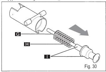
detach the rod (G) from the pin/gasket assembly (I);
