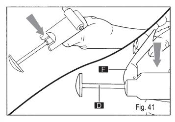
insert the mixer auger into its seating;
