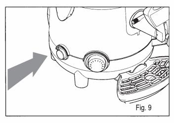
Set the thermostat to the required temperature to heat the product inside the how!
