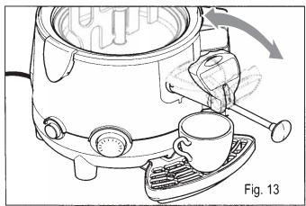
Fill the bowl with water and set the thermostat to 50°C (122°F). Operate the appliance for at least 15-20 minutes; increasing this amount of time will release any product residues that may be stuck to the sides of the bowl.
