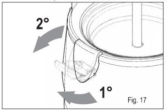
release the bowl from the machine body, using two fingers to prise it away from the fixed steel part of the mixer auger (A) and the others to grip the outer edge of the bowl (B): Gradually pull the bowl harder until it comes away
