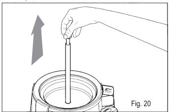
place the bowl on a flat surface and using both hands, romove the gasket by sliding it upwards in the direction shown by the arrow.
