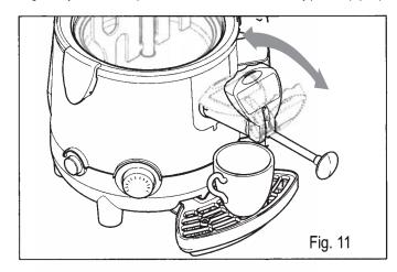
If the product is especially thick, it is advisable to keep the rod pulled out at the maximum position; any clogging in the dispensino line may be removed by sliding the rod back and forth while keeping the machine, as shown in the Fig. 12.
